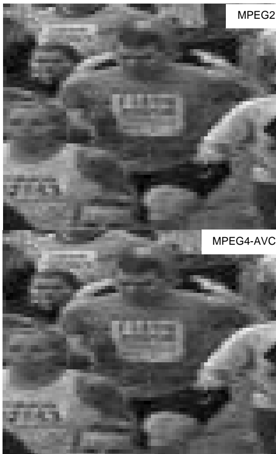
Fig. 8 artefact comparison between MPEG-2 and MPEG-4 AVC at 50Mbits.
